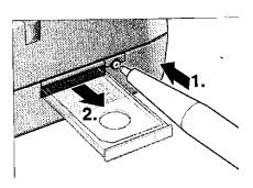
3. Insert the SIM card in the SIM card holder and push it back into the housing.
